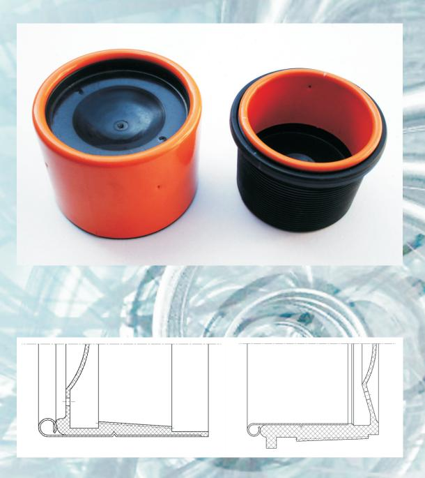
Protector (cap and nipple) for casing pipes, type LIFTABLE
