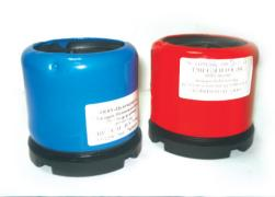
Thread protectors (cap and nipple) made of polyethylene, reinforced, non-reinforced and with steel shell for protection of tool joint thread of drill pipes produced to TU, GOST, and API Spec. DP, TU 2291-004-79238319-07.
